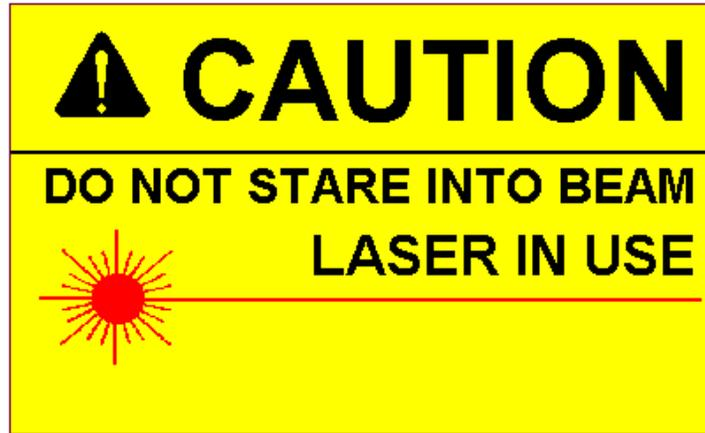
In accordance with ANSI Z136.1-2007, an area which contains a Class IIIb or IV laser or laser system shall be posted with an appropriate caution sign. (See example below)
